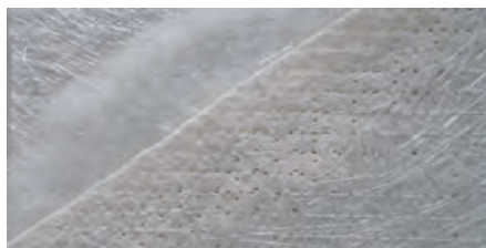
Spheretex’s Sphere Easy IP is described as an all-in-one solution and consists of four layers with the objective of reducing lamination weight and cost
