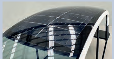
Panlite is a tough new transparent resin polycarbonate being used to protect the solar cells on the roofs of electric vehicles. The ability to curve this material, and its resistance to impact and UV fading (with a special coating) could make it ideal for future marine solar applications, such as on this Sunreef Eco 50
