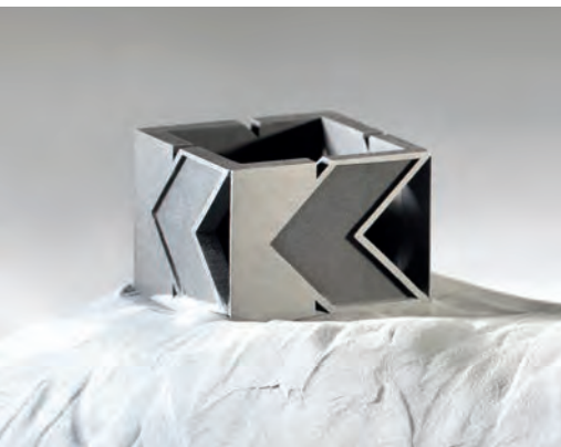
A part made from Stellite in a laser powder bed additive manufacturing machine
